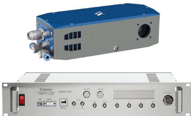
**MP1** pulse picker consists of built-in fast driver and a Pockels cell. This unit is able to select pulses at up to 600 kHz rate. **MP1** requires sync pulses from the laser for the driver control or can be used with **pMaster 4.0H** generator. In setup with **pMaster 4.0H** generator can be synchronized for single pulse picking from max 30 MHz repetition rate pulse train.
