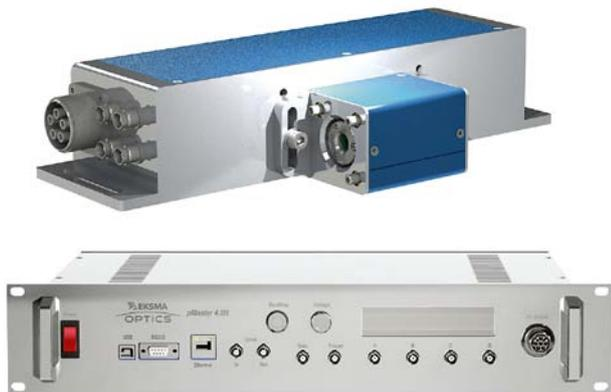
**UP1** pulse picker consists of built-in drivers in full bridge configuration and a Pockels cell attached to the unit. The **UP1** pulse picker in setup with **pMaster 4.0H** generator is able to select pulses at up to 1 MHz rate from max 100 MHz repetition rate pulse train.
