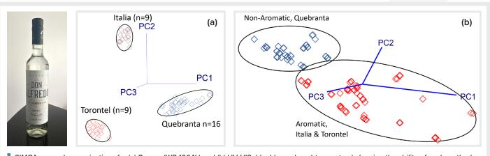
SIMCA score class projections for (a) Raman (WP 1064L) and (b) UV-VIS, (dual-beam benchtop system) showing the ability of each method to separate aromatic from non-aromatic grape varietals, and further discrimination of exact grape varietal by Raman spectroscopy.
