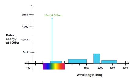
Tunable wavelength lasers are available at the following power and wavelengths:
