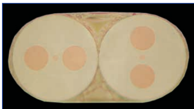
End Face Of Dual Fiber Assembly Showing Stress Rod Alignment
