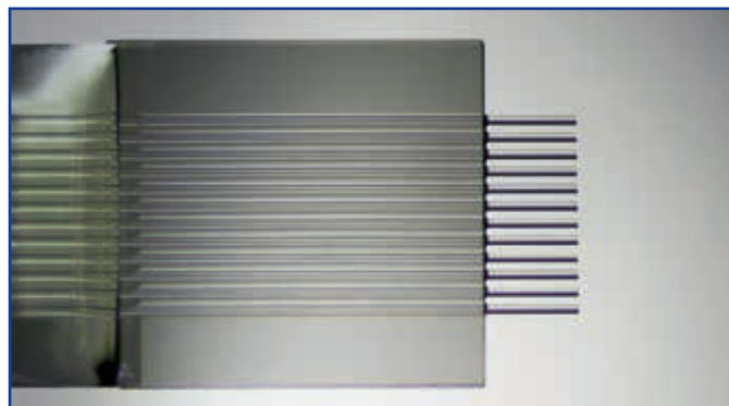
V-groove Assembly with polished/cleaved fibers with a Silicon v-groove substrate
